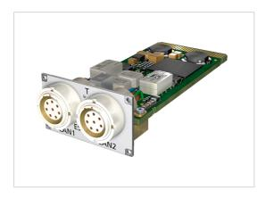
The two CAN interfaces can be configured individually into High Speed or Low Speed CAN buses. The High Speed bus is connected via the TJA1040 transceiver and the Low Speed bus via the TJA1055 transceiver.
