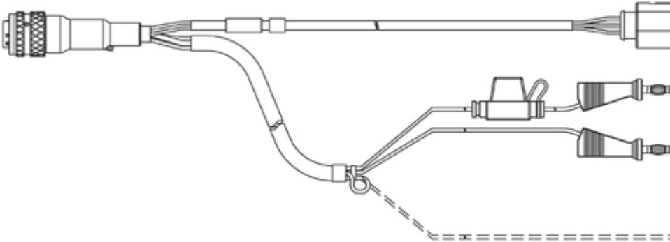
Lambda 센서 케이블 LSU 4.9, Souriau 8ST12-35 - RB150 (Code 1) - Safety Banana (22mc-6fc+2mc), 3 m
