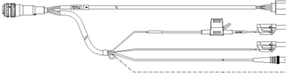
Lambda 센서 케이블 LSU 4.9, Souriau 8ST12-35 - RB150 (Code 1) - Banana (22mc-6fc+2mc), 3 m
