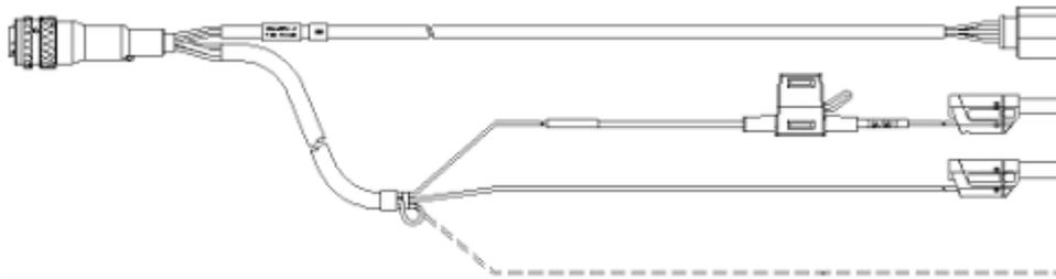
Lambda 센서 케이블 LSU 4.9, Souriau 8ST12-35 - RB150 (Code A) - Banana - BNC (22mc-6fc+2mc+2mc), 5m / 16.4 ft
