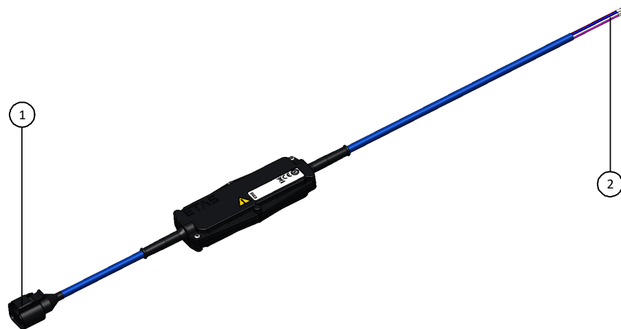
Fig. 4-2 Connections of the Smart Lambda Sensor Cable
