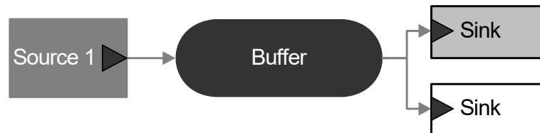
Fig. 3-25 Connection: One source, several sinks, different timing
