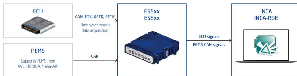
Figure 1-1: Setup for the INCA RDE Online Software: Connection
