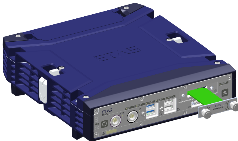
Fig. 5-4 ES820.1 with replaceable memory module
