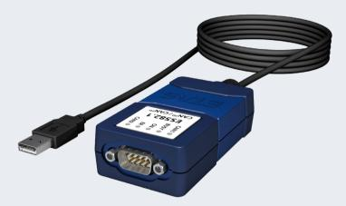
The ES582.1 module is a dual-channel. compact and cost effective CAN FD interface. The module is a solution with flexible data rate support for connecting the PC or notebook to vehicle CAN (Controller Area Network) busses or the CAN port of individual electronic control units (ECU) on the vehicle.
