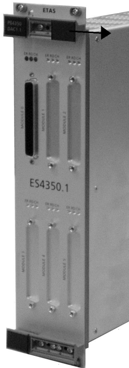
Fig. 1-4 Removing the Middle and Right-Hand Handle Covers
