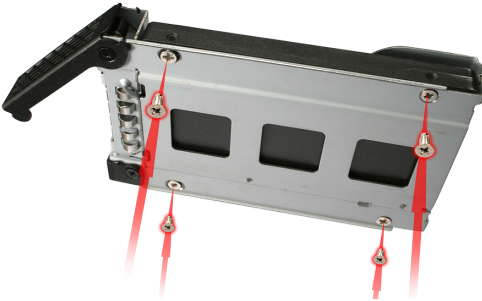
Figure 05.2: Mounting a drive into the tray
