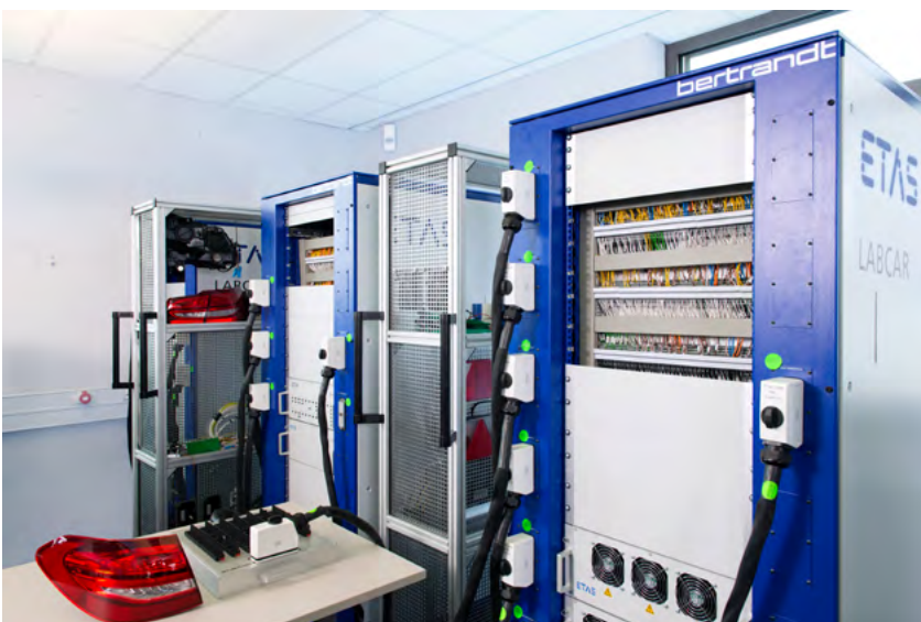
Fig. 3: HiL testing of the “tail lights” components of the “lighting” subsystem.
