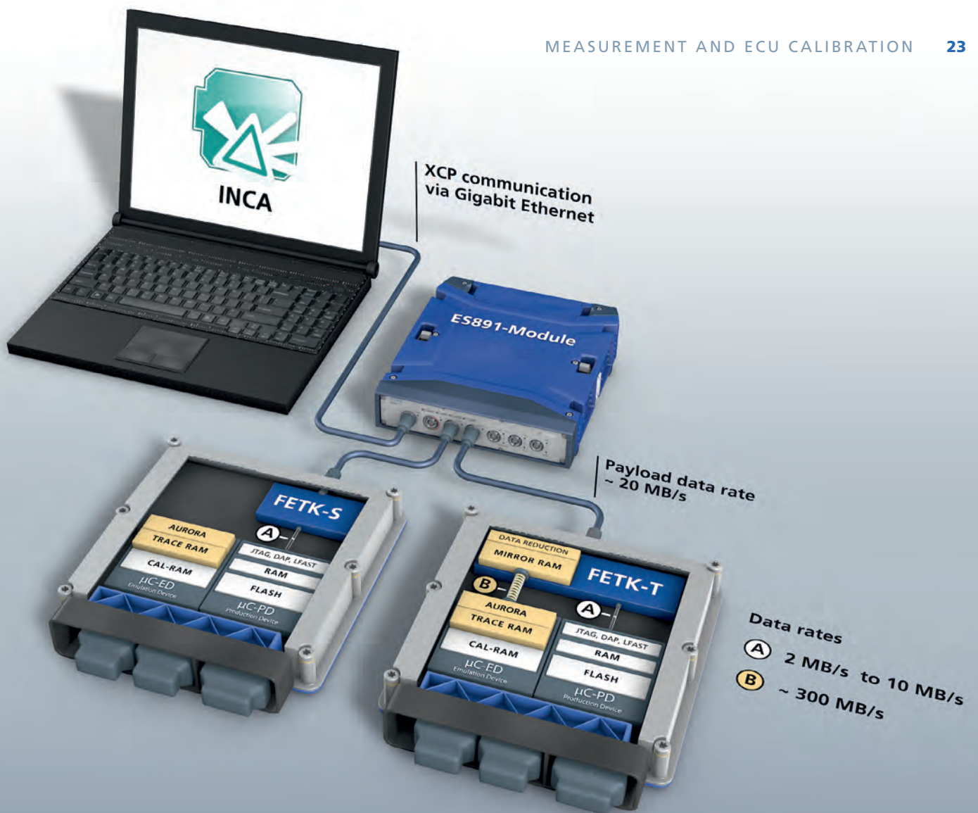
Figure 2: Acquisition of data from the ECU through the FETK interface. FETKs are offered in two versions, FETK-S (left) and FETK-T (right). Both variants use a microcontroller-specific production device ( \mu C-PD) debug interface such as JTAG (Joint Test Action Group), DAP, or LFAST as control access. Additionally, T-type FETKs support the particularly powerful \mu C emulation device ( \mu C-ED) trace interfaces, along with the high-performance transmission of trace data from the ECU over the serial Aurora interface.
