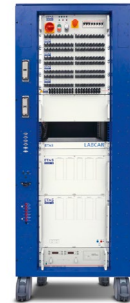
Figure 1: Front view of a fuel cell HiL system.
