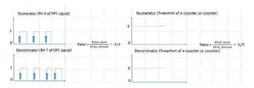
EATB detects the situation based on the number of signals you provide. Therefore, you cannot mix "bit" and "int".
