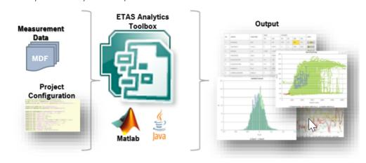
The data recorded and uploaded to some storage location on a server can be transferred to EATB. EATB provides a visualization of the relevant information and critical threshold violations.
