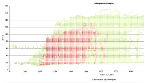
In this example, the engine speed (nmot) is shown on the x axis and the air charge (rl) on the y axis. The plot also has a child shown in red. The red points are the data points when the engine is running in half-engine mode. The green points are the data points when the engine is running in full-engine mode.
