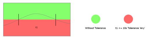
If the signal time series enters the yellow range > 10s continuously, the traffic light is yellow.
